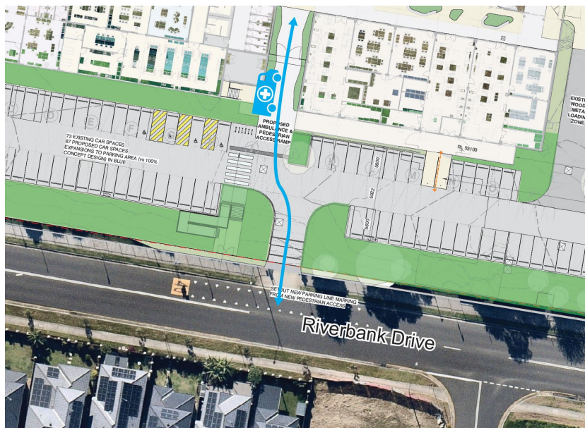
Figure 5-4 Emergency (ambulance) access to the oval
